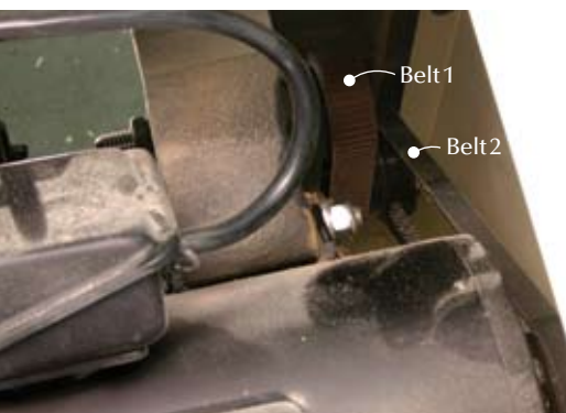
A two-for-one deal. The "two-step pulley system" on the Jet and General saws helps to increase blade speed and reduce overall vibration of the machines.
