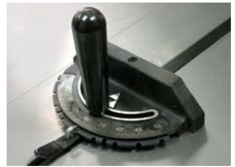
Plenty of stops are a positive. The Delta miter gauge rated number one. By pressing the spring-loaded lever you can adjust to any one of 11 positive stops, or locate the pointer to the desired angle setting and tighten the handle for a firm hold. This gauge was snug to the table-saw slot exhibiting no sloppiness.
