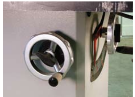
Put the lock where the wheel is. Steel City, along with Craftsman and Delta, has the inner hand wheel locks for both the blade height and tilt adjustments. They're easy to use and conveniently positioned.
