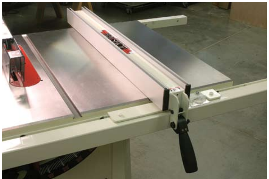
Best fence, period. The Jet fence was outstanding. It slid like a bobsled at the Olympics. The aluminum fence faces have a T-slot for adding jigs or fixtures. When locked, the fence held tight to the table.
