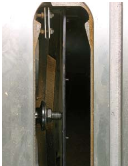
A just-missed design. Looking into the insert area of the General saw, you can see the blade shroud. You can also see the small offcut caught in the shroud. A zero-clearance insert would keep that offcut out, but neither of the inserts shipped with the saw can.
