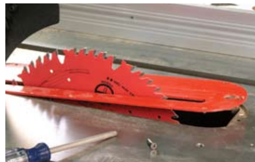
Double jeopardy. Two aggravations are shown on the Grizzly saw. First, the insert plate is very thin at 1/8" and there's no reinforcement on the bottom of the plate. Second, table insert screws require an extra tool close at hand. This saw uses the screw to hold the plate down and flush.
