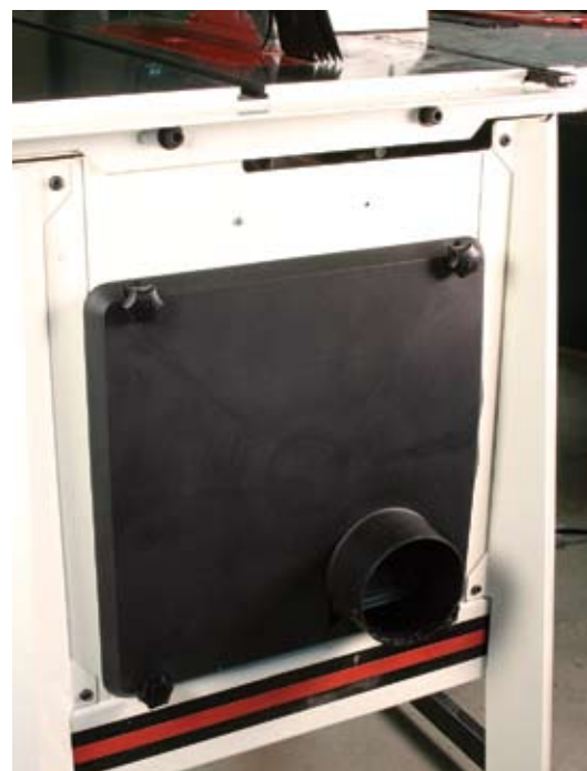
Where are the hinges? The access door on the Jet is not a door – it’s called a “dust hood.” It’s held in place with small lock knobs and is something I’d change if this saw was in my shop.
