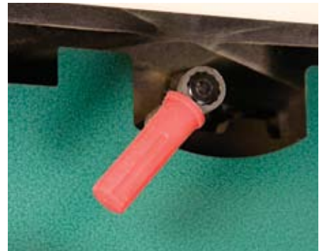
Aggravating lock lever. The General, Jet and Grizzly saws use a lever located front and center to lock blade-tilt handwheel. The location makes these levers inconvenient to use.
