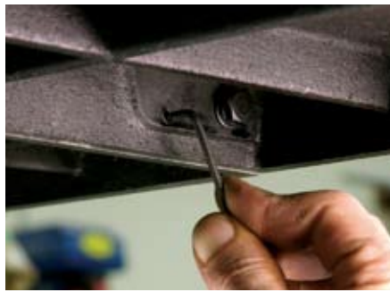
Set up to work fine. Set screws added to the wings of the Steel City saw made for accurate adjustment of the wings. A level tabletop was an easy task out of the crate.
